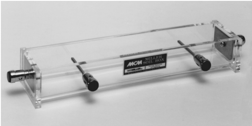
Figure 6.25 Soil resistivity box. (Photo courtesy of M. C. Miller Co.)
