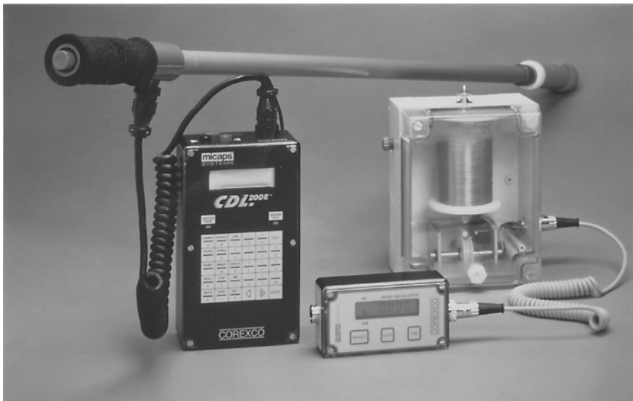
Figure 6.26 Close interval survey equipment. (Photo courtesy of Corrpro Companies, Inc.)
