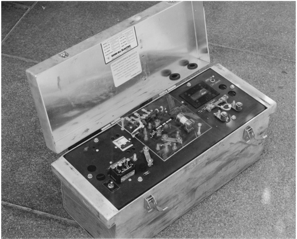
Figure 6.17 Portable test rectifier. (Photo courtesy of Corpro Companies, Inc.)
