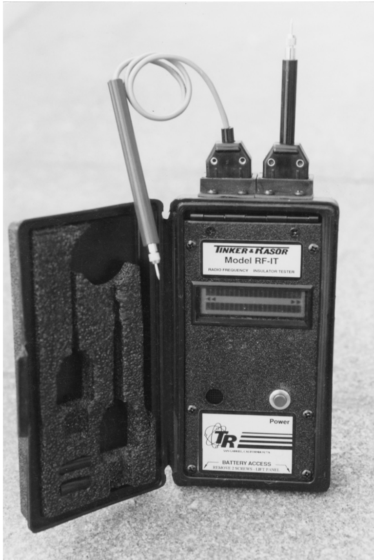
Figure 6.16 Insulator checker. (Photo courtesy of Tinker and Rasor.)
