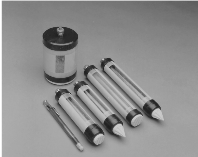
Figure 6.19 Portable copper-copper sulfate reference electrodes. (Photo courtesy of M. C. Miller Co.)
