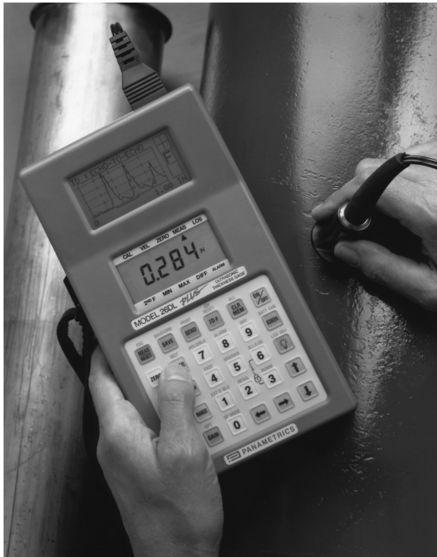
Figure 6.9 Ultrasonic wall thickness gage. (Photo courtesy of Panametrics.)
