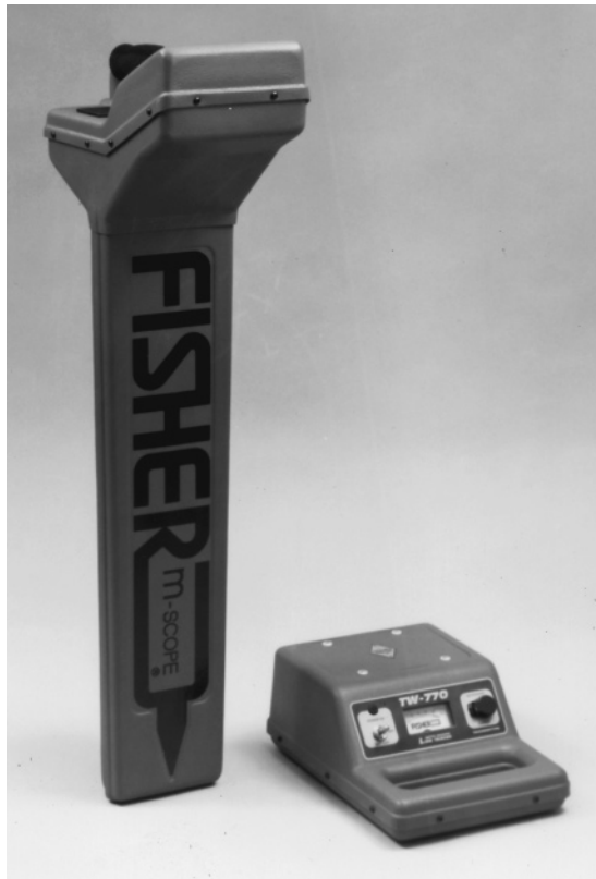
Figure 6.13(b) Pipe and cable locator. (Photo courtesy of Fisher.)
