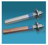
In operation, the copper anode produces ions which are carried by the flow of seawater, creating an environment in which barnacles and mussels will not settle or multiply. By introducing copper ions in very small concentrations, around 2 ppb, the Impressed Current Anti-Fouling
